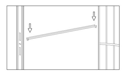
**Step 4** Screw through the stud work at the rear of the pocket into the rear pocket vertical (a pair of screws every 50cm)
