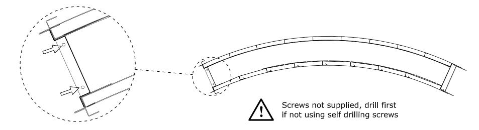
**Step 6** Fix the top rail to the stud work above the rail by drilling holes in the outer wings of the rail and screwing into the stud work. If you are using wooden stud then a screw each side every 40 cm. is adequate. If using a cut metal stud to obtain the curvature it is recommended that each cut section is screwed to the top stud work.
