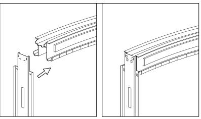
**Step 3** Centralise the frame between the stud work and check for alignment by looking down a sight line between the vertical of the metal door post and the edge of the pocket entrance, these two vertical sight lines should be PERFECTLY parallel. Screw the metal door post through the metal doorpost (a pair of screws every 50cm) to it's side of the stud work ensuring it is EXACTLY plumb and checking the sight line at all times.
